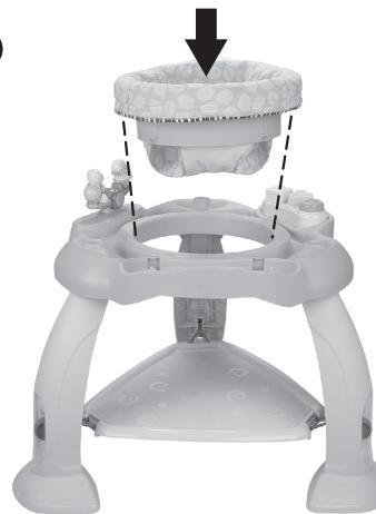
Place the seat into the play surface. Ensure that the four highlighted tabs slot into the inner rim of the surface. The seat carrier should rotate freely within the play surface. The Seat Carrier should be fully seated to avoid being easily pulled out of
