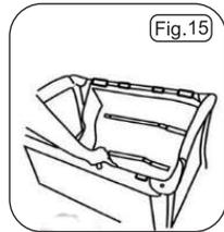
**Make sure all 12 clips are securely attached to the top rails**
