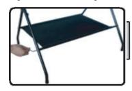
2.Connect the top assembly with the leg sets.
