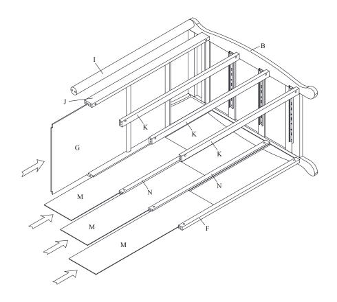
Step 9: Attach Back Cross Beam (C), Back Middle Rail (N), Back Bottom Rail (F), Top Round Rail (I), Front Cross Beam (J) and Drawer Rail (K) to Left Side Panel (A) using 9 Bolts (#2) and 9 Barrel Nuts (#3) and 7 Wood Dowels (#4). Tighten firmly with Allen key (#1).
