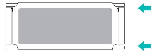
Pass the upper and lower rails through the mesh panel. When installing the mesh panel, the side with zipper and warning faces outwards.
