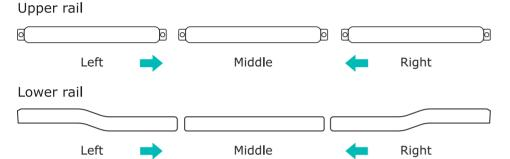
Connect the left, middle and right rails in order until the button pops out from the slot.
