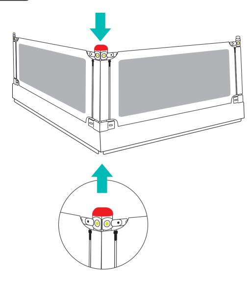
If multiple bed guardrails are installed in combination, there will be gaps between adjacent bed guardrails. Please tighten the two bed guardrails and fix them with L-shaped buckles. After assembling, if the fence shakes a lot, you can fix it to the bed with screws.
