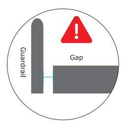
If there is a obvious gap between the guardrail and the mattress, it is evidence that your installation is not in place or the mattress is not thick enough.
