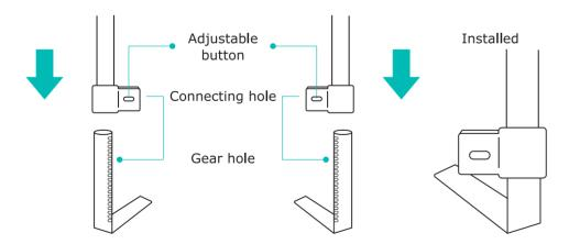
Connect the left & right lifting rod with the left & right L-shaped base in the direction as the arrow.
