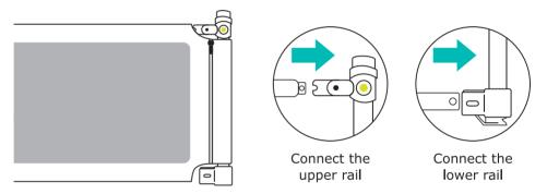
Insert the rail into the slot until the button protrudes from the slot, and the zipper or printed side faces outwards.
