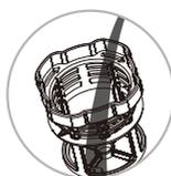
2. Rinse the filter cup and filter with water.
