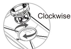
3. After rinsing the filter cup, put it back to the dishwasher and turn it clockwise to fix it until the triangle sign on the filter cup matches the sign on the stainless filter.
