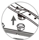
1. After removing the bowl basket, pull the lower spray arm up to get rid of the buckle.
