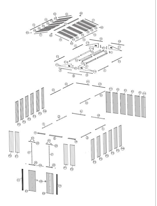
Assemble base bars from (1) to (4R) with (F1) Screws. Then place the entrance taper channel (5)on top of the bar(3L) and(3R). Secure with (F1) screws to the foundation. Seeing the following figures. Make sure the base bar assembly in a perfect square.
