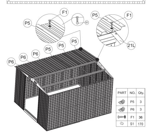
Place the roof panels (P5),(P6) on the top of Gable panels and roof supports Line up the boles and secure with (F1) bolt and nut with washers.
