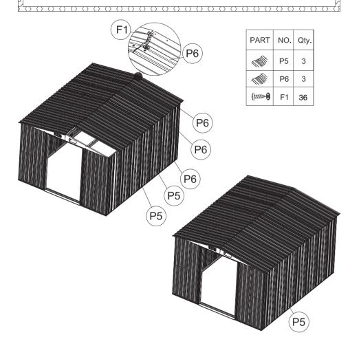
Assemble the roof flashing (15) and (17),(18) with roof panels secure with (F1) screws with washers. Then place 4 piece of top corner (GC) on the roof flashing joints. and secure with (F1) screws with washers.
