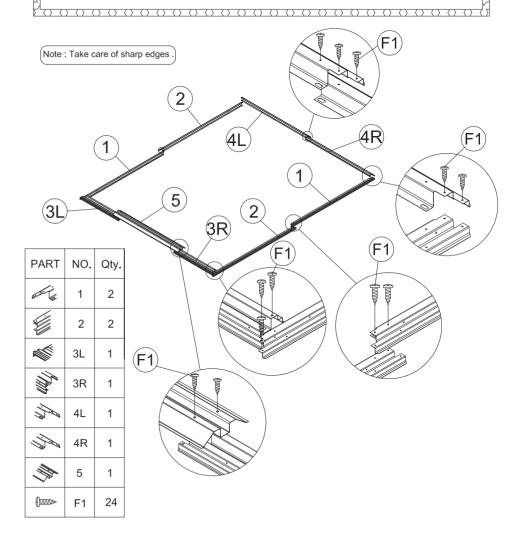
Place the wall panel (P1) and (P2) on the base bar (3L) (3R),(4L)and (4R) as showing .Side wall of the shed line up the Holes With base bar.Secure with (F1). Screws with washers from outside.
