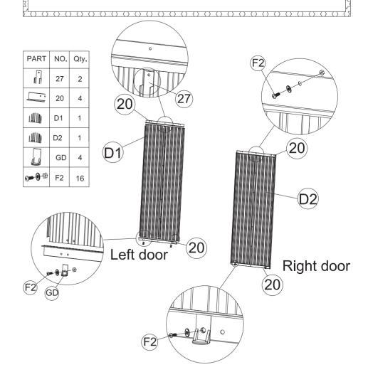
Fix 2 pieces of the door handle (D2) to door panels from inside with (F2) bolt and nut.
