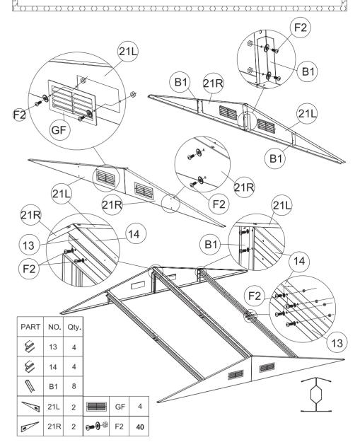
Place 4 piece of the Gable panels (21L) and (21R) (13) (14) on the top of the sliding channels (7).(8) and back top bars (10L).(10R),Align the holes and secure them with (F1) screws from inside as showed.
