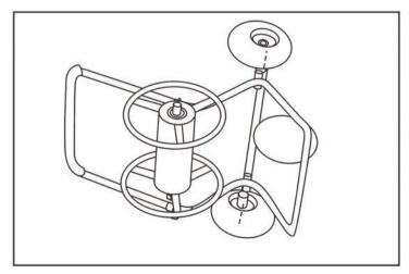
For right-handed users, hose reel (7) should be facing the same way as in the picture - with crank slot (7-a) on the right (far) side, left-handed users may reverse the hose reel. Line up holes in hose reel (7) and frame (1), and also make sure the U bracket (14) attach to the frame (1) by using four Carriage bolt (8), small washers (15) and lock nuts(10). Tighten the nuts to secure the hose reel (7) to frame (1), this will also secure the pull handle (6).
