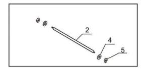
B. Slide wheels (3) -hub facing in, air valve facing out onto each end of the Axle (2), then attach large washers (4), large nuts (5), tighten with wrench to secure
