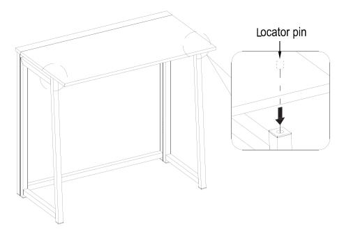
3. Gently lift up the desk top panel a little so that the locator pins underneath the top panel align with the top holes of the side frames properly. Press down the top panel evenly to ensure both locater pins are fully seated.
