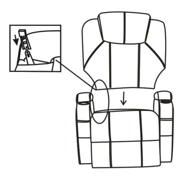
Turn over the base part, you will find the power wire and remote wire are binding by three cable ties. Please cut off the #2 cable tie and keep #1 & #3 to fix position.
