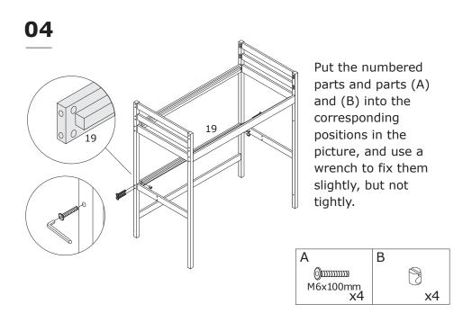
Put the numbered parts and parts (A) and (B) into the corresponding positions in the picture, and use a wrench to fix them slightly, but not tightly. 10 A В M6x100mm **x4**
