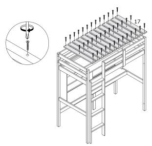
Install the parts(L) into the corresponding positions of the picture. Keep two ends fixed on the parts 15 on both sides, and the middle fixed on the part 16. Tighten the screws with the wrench.
