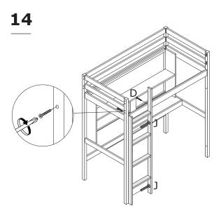
Use parts (J) to fix the part 2 to the bed leg, and then use part(D) to fix part 4. Be careful not to install them in a wrong position.
