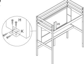
Use the metal plates (K) and screws (H) to connect part 20 and part 19 in the middle.
