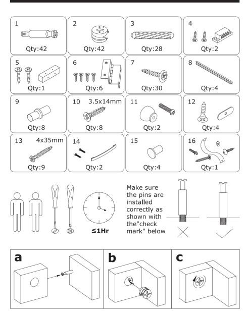
Below shows how the pins are used to assemble the panels together.
