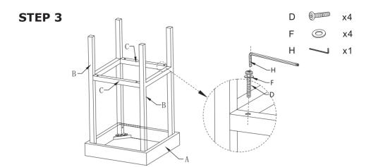
Tighten the assembled parts B,C using bolts (D) and washers (F).
