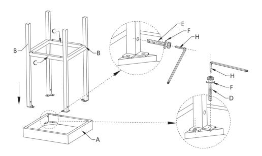
Lay seat (A) down on a flat surface. Attach assmbled parts B, C to the seat (A) using bolts (D), washers (F), allen key (H) in vertical direction.
