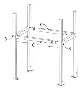
Attach frame (B) into stretcher (C). Please do not screw at this step.
