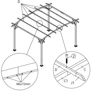
Turn the screw-mounted side towards the ground
