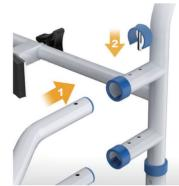
Step 3: Detach the small plug, nut and arc sheet from the adjustment shaft.
