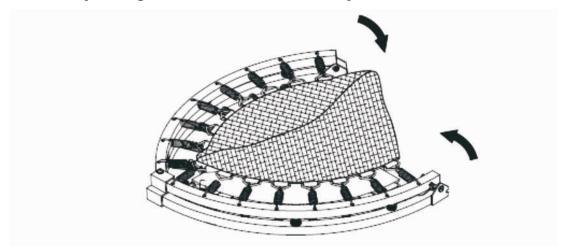
7) Insert the secure pin at the end of the frame where the rails connect.
