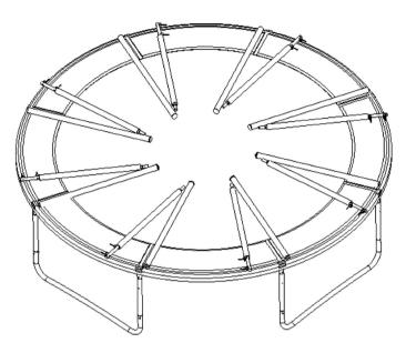
2. Attach the lower tube to the frame of trampoline using the quick clamp.
