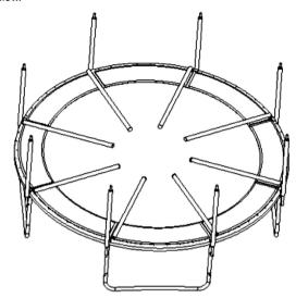
4.Fit the upper pole(with the netting )into the lower pole, as shown below, then sliding net down the poles.
