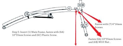
Fasten (6A) 10\*55mm Screws and (6C) Plastic Screw.
