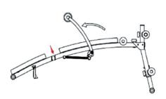
Step 1: Unfold (1) Main frame and Insert (10) 8\*55 Bolt to the joint. Stabilize it with (9) M8 Plastic Screws. And fasten (12) Handgrip with (13) 8\*35mm screws.
