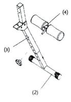
Step 3: Insert (4) Lower Roller Pad to the hole of (2)&(3), Fasten it with (6C) Plastic Screws. The height can be adjusted.
