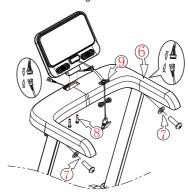
As shown in step 6 and 7, turn the upper cover of the armrest downward to buckle with the riser (be careful not to press the signal wire on the right riser) to align the mounting holes. Use M8\*16 hexagon socket pan head screws and two 48 washers to lock the armrest assembly parts on the left and right risers respectively.
