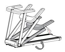
Take the main machine out of the carton box and lay it flat on the carpet or soft cushion. As shown in step ①② in the figure above, lift the left and right riser upwards, ②③use the supplied tool "6mm Allen key" to tighten the screws clockwise. Lock the left and right risers to the frame. Then install the riser covers as shown in step ④⑤; use the countersunk self-tapping self-drilling screw 4.2×16 to install the lower cover of the riser under the left and right risers.
