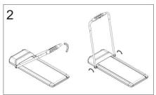
Step 2: pull up upright tubes to proper position, then fasten the knob at both bottom side of upright tubes.
