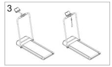
Step 3: Insert IPAD holder and put safety key on panel. All assemble finished.
