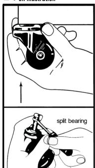
If caster assembly fits loose, using a screwdriver, slightly spread apart split bearing on shaft. If caster is difficult to insert, crimp split bearing slightly with pliers. Make only slight adjustments until caster fits properly.
