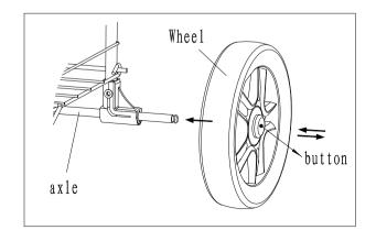
Once the wheel is attached to axle, push the button in while gently pushing down then release the button and push up ensuring it snaps on.
