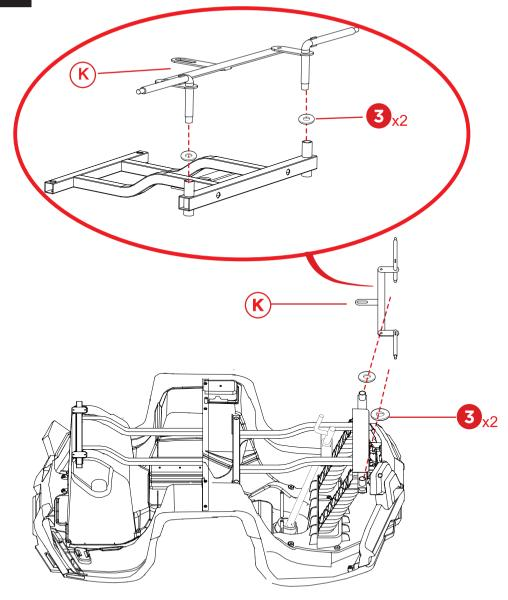
2 Lock Steering Bracket Gasket Nut Fixation
