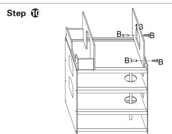
Insert B (2 pairs) screw in No.13 and No.9 panel, then lock it together.
