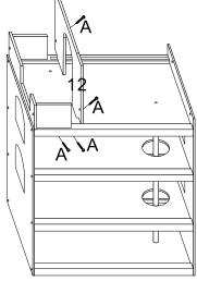
Use A screw to lock No.12 panel on No.5 panel, use A screw to lock No.12 panel on No.10 panel.
