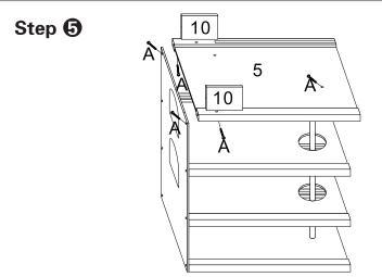
Use A screw to lock No.10 (2pcs) on No.5 panel, use A screw to lock No.5 panel on No.1 panel, use A screw to lock No.18 (bar) on No.5 panel.
