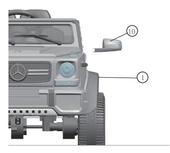
Figure 8: Install the rearview mirror (10) on the left side
