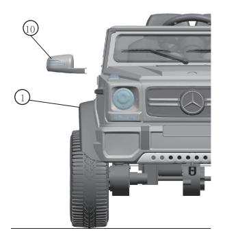
Figure 9: Install the rearview mirror (10) on the right side
