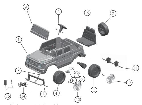
Assembly of your new car is simple, provided you carefully follow the detailed diagram and refer to component part numbers to ensure they are fitted in the correct order as shown above.
