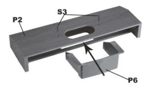
Insert the ball box into the card slot, align the screw holes, and then fix it with screws.
