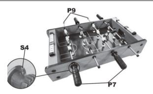
Install the handles and safety end caps at both ends of the teams, as shown in the figure. After pressing in place, lock the handles with screws.
